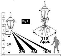
To avoid damage to the unit do not aim sensor towards the sun.
