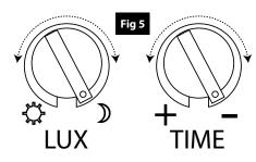
**ADJUSTING THE DURATION TIME:** the length of time that remains switched on after activation can be adjusted from  $(10\pm5)$  seconds to  $(4\pm1)$  minutes; rotating the TIME knob from (+) to (-) will reduce the duration time.
